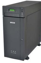
All libraries can be loaded and unloaded by using the removable 35-slot magazine. Single media im- and export can be done by using the extra mailslot in each Library. The optical drives, based on industrial standard, are very reliable Libraries and are able to write / read all types of optical media like DVD, BD and BD-XL.
