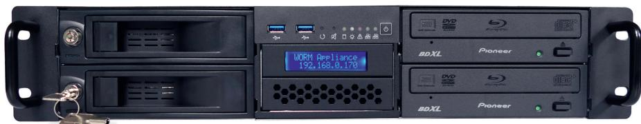
for example that a new medium must be inserted are sent automatically. If an optional second drive is installed media copies for offline archiving can be made in parallel. The internal data buffer is mirrored on a second hard disk (different manufacturers) providing a maximum of data security against data loss. If there should be a disk failure, the system will fix the error using its self-monitoring-functions (High Secure Protect). This function will write not
